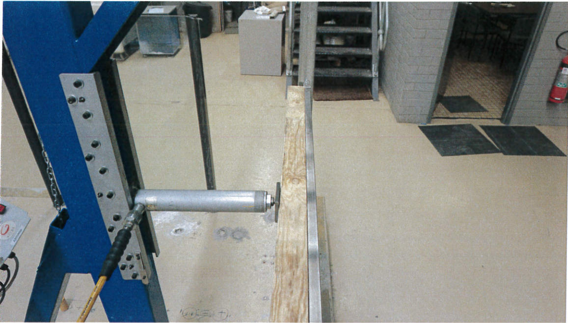
Figure 6: Horizontal Uniform Load - 750 N/m
