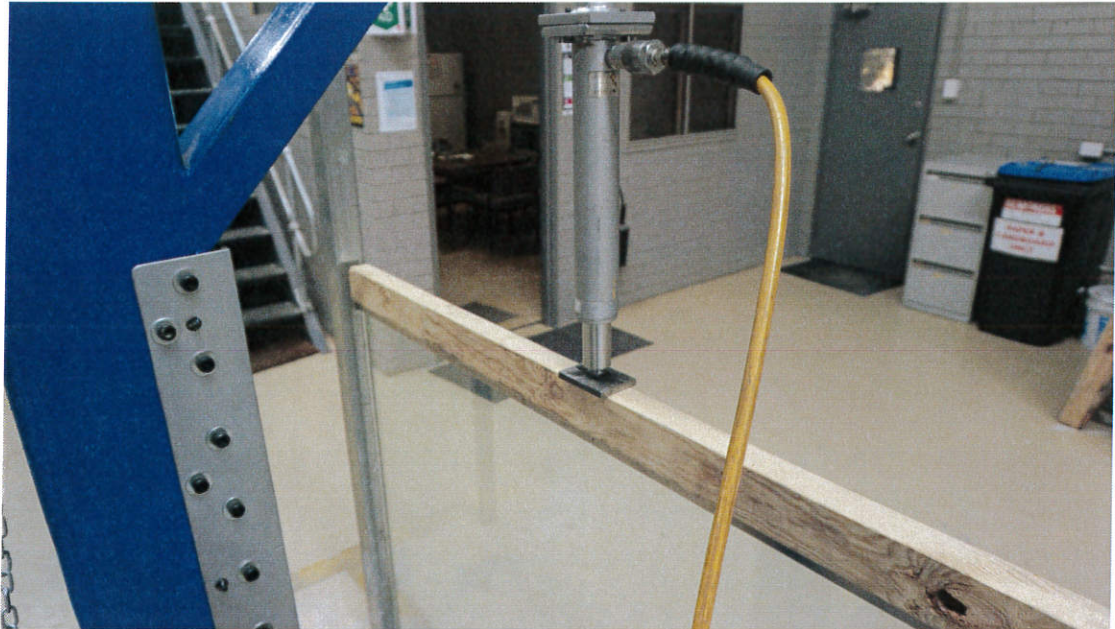
Figure 5: Vertical Uniform Distributed Load
