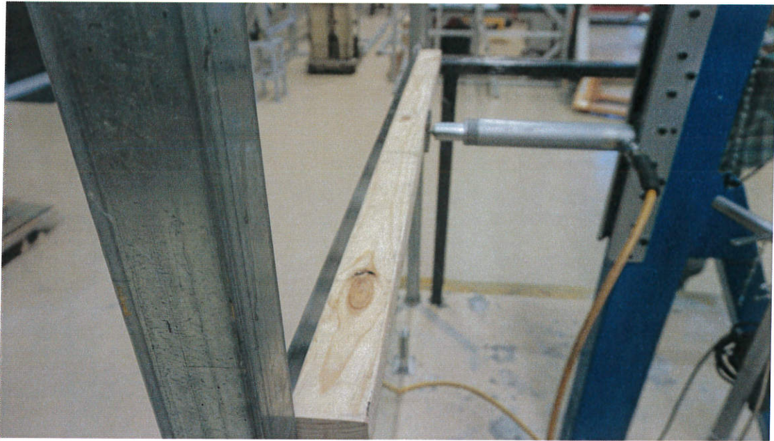
Figure 6: Horizontal Uniform Load - 750 N/m
