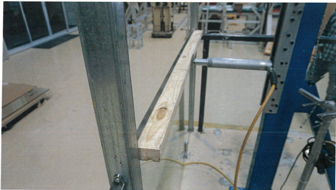
Figure 7: Horizontal Uniform Load - 1500 N/m
