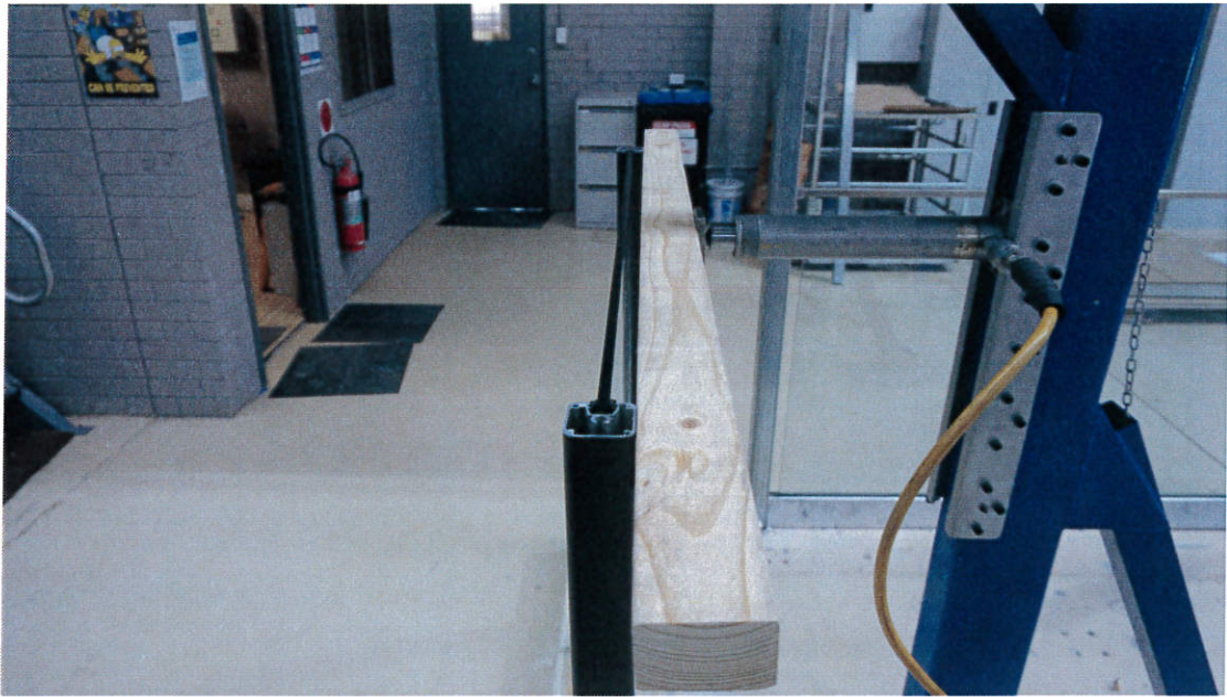
Figure 5: Horizontal Uniform Load - 350 N/m
