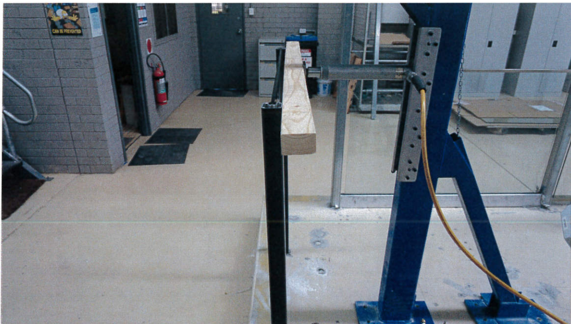
Figure 6: Horizontal Uniform Load - 750 N/m
