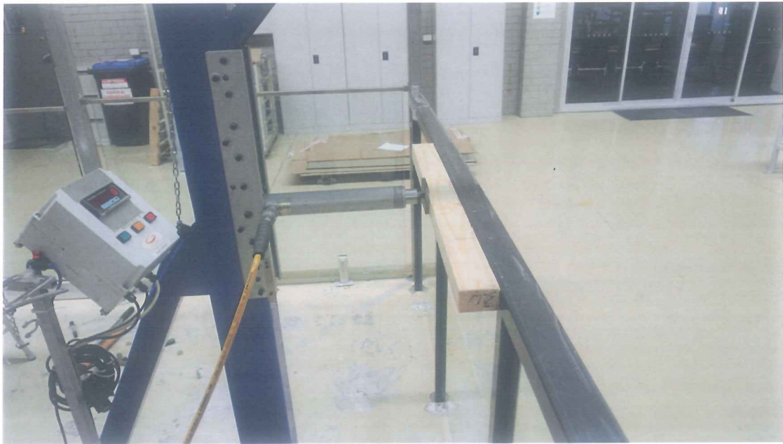
Figure 5: Horizontal Uniform Load - 750 N/m
