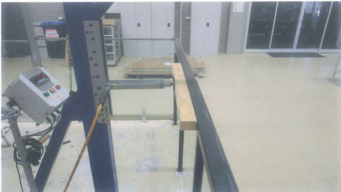
Figure 6: Horizontal Uniform Load - 3000 N/m
